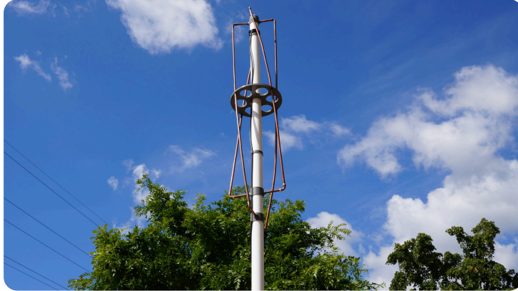
DIY Quadrifilar Helix Antenna
